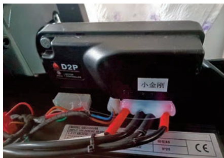
Area motor drive controller
